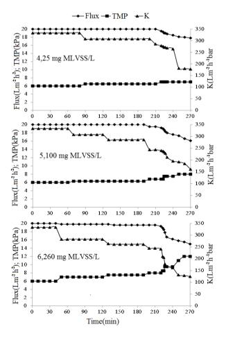
**Figure 4:** Behaviours of flux, TMP, and permeability in sub-critical conditions at short-term MBR operation
