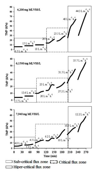
Figure 2: Performance with different MLVSS in MBR systems: critical and sub-critical flux
