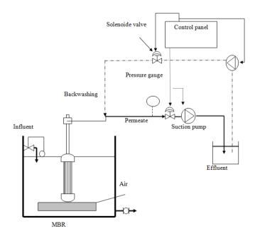
Figure 1: Schematic diagram of the laboratory-scale MBR system
