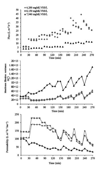
Figure 3: Performance with different MLVSS in MBR systems: critical and sub-critical flux
