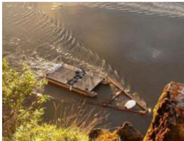
Figure 18. Debris boom protecting surface turbine (Tyler 2011)
