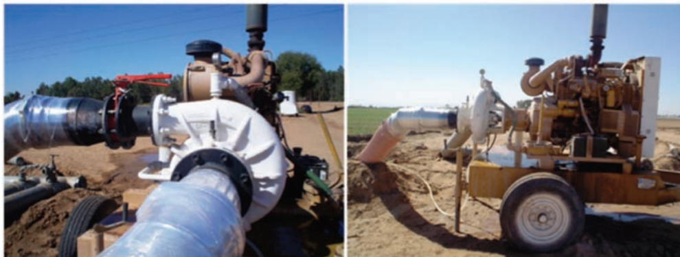
Figura 4.14. Motobomba centrífuga diesel remolcable.
