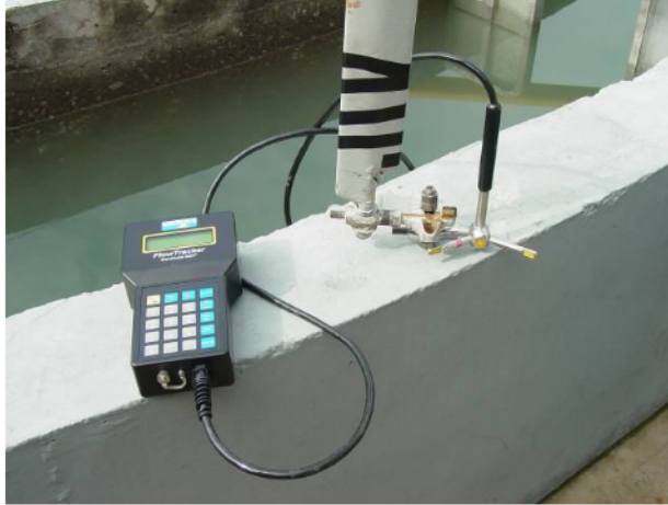
(c) Velocímetro Doppler usado (modelo "FlowTracker", marca "Sontek / Ysi")
